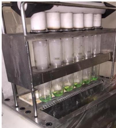
**ANEXO 9-F. Adición de agua destilada a cada tubo de digestión**
